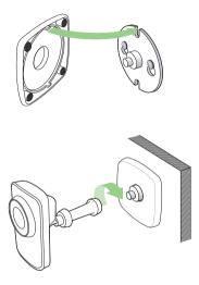
Align base with plate and screw on camera post.
